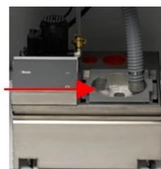
A Static filter unit
