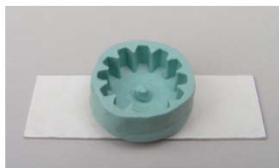
RepliFix replica of gear wheel, mounted on Backing slide
